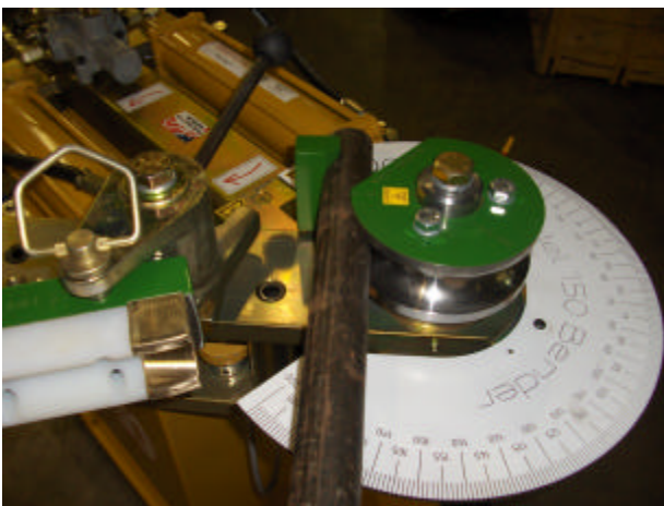
Figure 8 Inserting material to start bending
