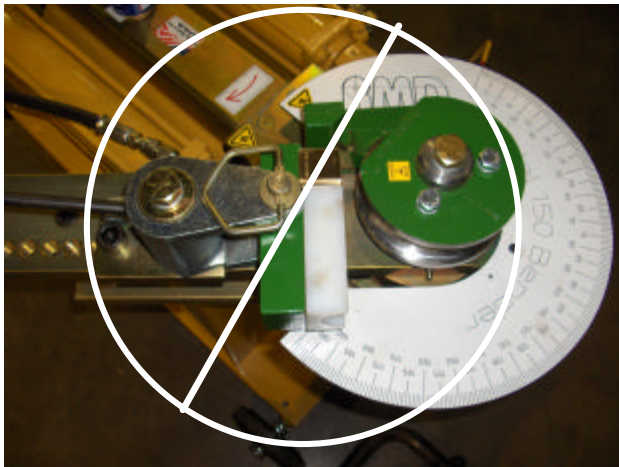
Figure 5 Incorrect counterdie position (Too far away from die)
