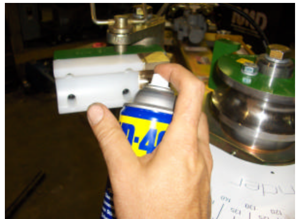
Figure 9 Lubricating counter die
