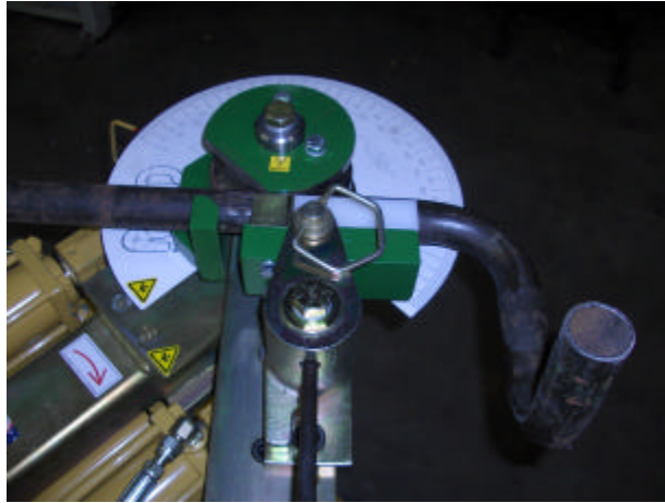
Figure 19 Not enough material to complete the bend without crashing
