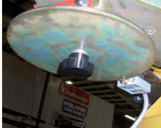
Figure 13 Autostop adjusting knob
